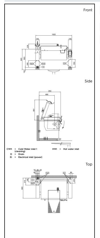
Electric Supply voltage: 400 V/3N ph/50/60 Hz **Total Watts:** 20.6 kW Water: Drain "D": 1/2" Installation: FS on concrete base;FS on feet;On base;Standing against wall Type of installation: **Key Information:** Working Temperature MIN: 50 °C 250 °C **Working Temperature MAX:** Vessel (rectangle) width: 1050 mm Vessel (rectangle) height: 326 mm Vessel (rectangle) depth: 558 mm External dimensions, Width: 1600 mm
